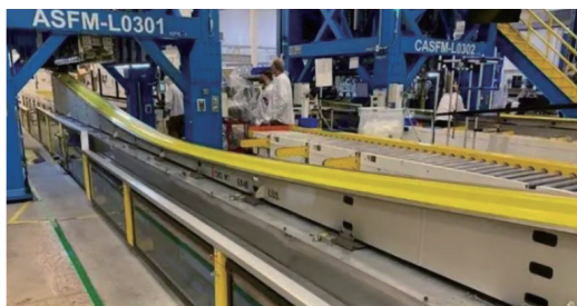
(a) Automated stiffener forming machine for producing thermosetting stringers
